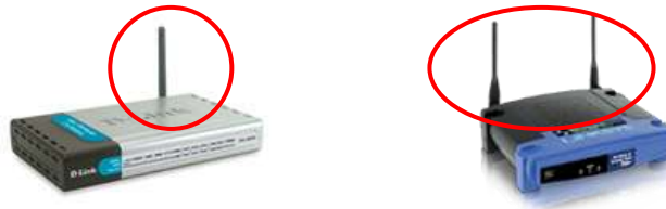
Figure 1, D-Link (left) and Linksys (right) broadband modems with built in wireless access point
